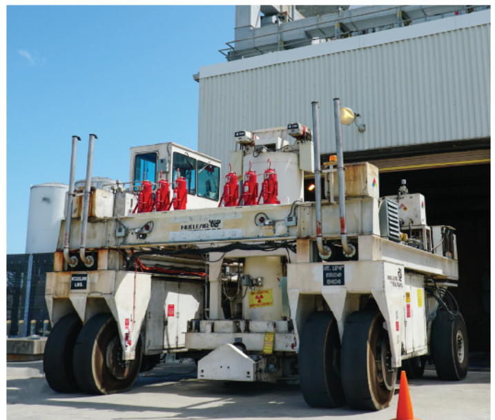
The Shielded Canister Transporter is used to move filled canisters to storage inside the Glass Waste Storage Buildings.
