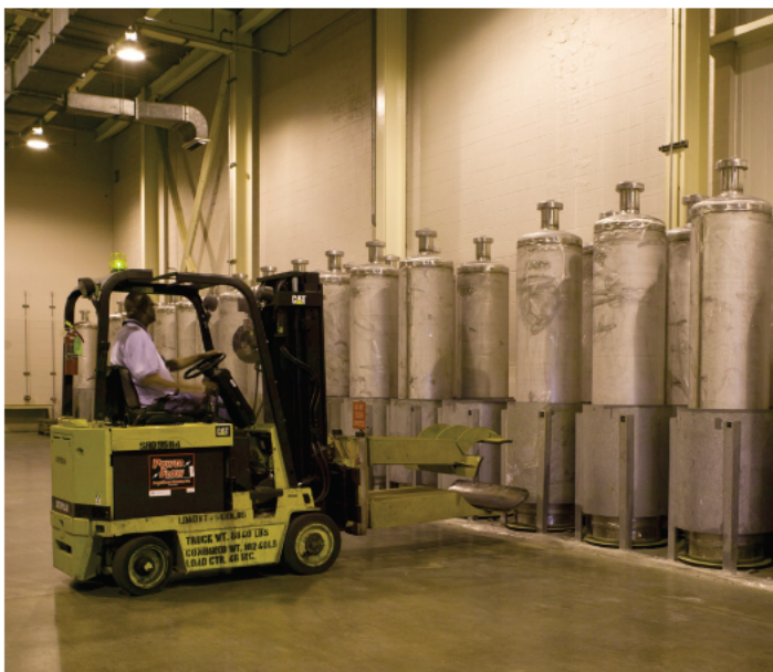
Workers use a special forklift to move an empty canister for its inspection at DWPF. The canister will be filled with vitrified high-level waste.
