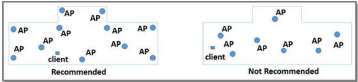
Figure 4: Recommended AP Placement
