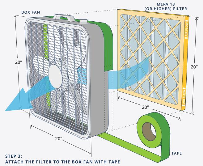
Once the box fan and filter are correctly positioned (the front of filter is placed squarely against the back of fan), use tape to attach them together on all four sides. Apply enough tape so that the filter is securely attached to the fan and the seam is continuous with no gaps. Clamps, bungee cords, or string may also be used in the absence of tape. Sealants and wet glues are not recommended as they may be an additional source of VOCs in the room and may complicate filter replacement.
