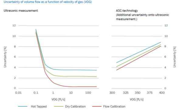
This exemplary uncertainty statement according to GUM (Guide to the Expression of Uncertainty in Measurement): ISO/IEC Guide 98-3:2008-09 shows a F1F-S in 1-path, 16" nominal pipe size configuration and assumes a gas temperature of 68 °F, ambient pressure, a typical molecular weight of greater than 27 g/mol.
