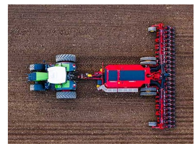
The Väderstad Tempo L 16-24 Central Fill pulled behind a tractor both seeds and fertilizes in a central bulk system.
