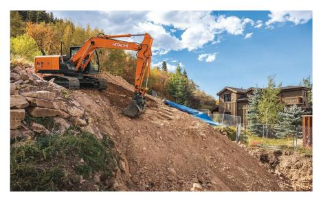
tightly to the slope. On the other hand, triple-bar grousers are good for flat and reasonable slopes, but they may slide once you begin work on 1-to-1 ratio slopes and other steeper jobs.
